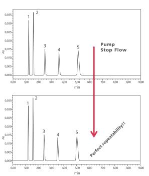
Fig.8 Stop-flow test under 100 % aqueous mobile phase conditions
