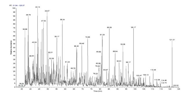
Identified unique proteins, peptides and average Full Width at Half Maximum (FWHM) from 200 ng Hela Tryptic Digest injection on an SenSil C18-AQ, 1.6 µm, 250 mm x 75 µm ID column using different gradient lengths. Samples were run on a M-class UPLC coupled to a Bruker timsTOF Pro, dia-PASEF acquisition. Data analyzed using DIA-NN.
