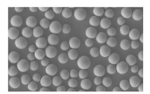
Fig.2 TEM image of 3 particle size silica gel
