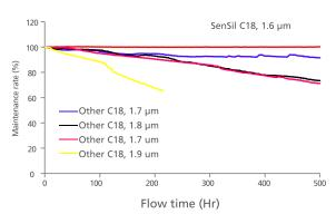
Fig.3 Retention time maintenance rate with respect to liquid flow time
